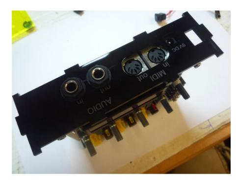
2:) then the underside is put into the recesses of the rear side. Make sure that the drill holes match the holes of the spacers. Then the base plate can be screwed down with 4x M3x6mm screws.
