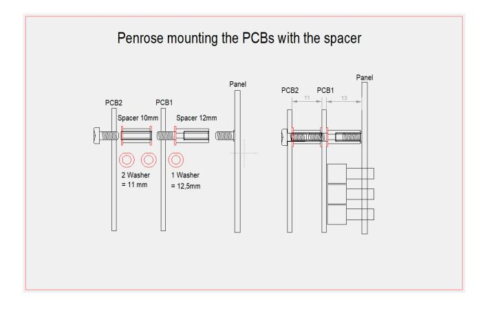
If 10 mm and 12 mm spacer are in the kit, mount the pcbs like in the picture above
