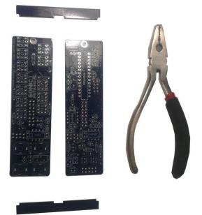
First take the PCB and separate it using a pair of pliers.
