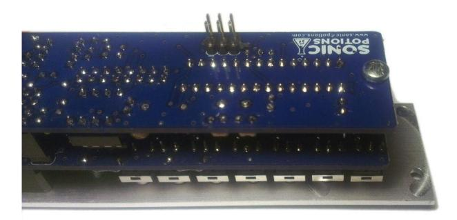
Make sure the 3 electrolytic capacitors do not touch the upper PCB!!!
