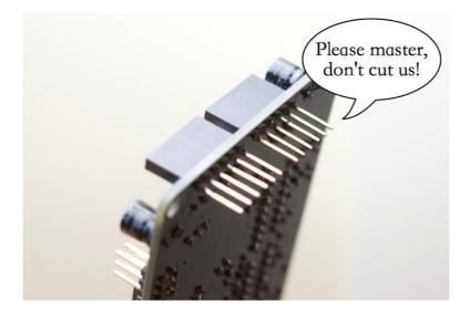
Do not trim the leads of the board stacking connectors. You might have gotten this habit if you have built Shruthi-1s... Don't do it! The voicecard is stacked on top of the motherboard, so the 6 leads of the 1x6 connectors should be kept. This is the same stacking approach as the Arduino "shields".
