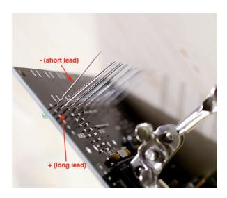
Add the LEDs. They are polarized, the shortest lead and flat side of the LED (-) are on the side of the switches; the longest lead and rounded side of the LED (+) are on the side of the resistors. Note that the colors and types of LEDs vary from batch to batch of kits – but no matter how they look, they need to be soldered the same way!
