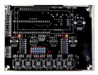
The 220R resistors soldered at this step are current-limiting resistors for the LEDs - they set the brightness of the LEDs. The 220R value printed on the circuit board is suitable for standard low-intensity green, yellow or red LEDs - and a lower value could indeed damage the LEDs. For blue or white LEDs, a higher value, such as 1k, must be used.
