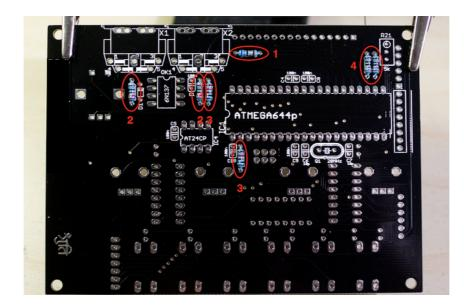
First, we will populate the bottom side of the board – starting by the shortest and smallest parts. Add the following resistors:
