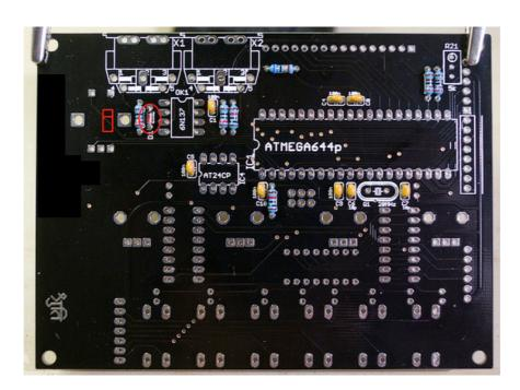
Finally, add the diode D1, which is **polarized**. The black ring of the diode should point towards the MIDI connectors.
