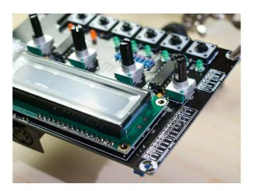
If all sounds good, insert the 16x1 connector between the LCD module and the PCB, and solder it first to the LCD module, and then to the main PCB. Be careful and keep the module aligned with the PCB!
