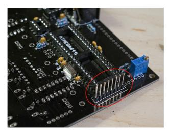
The connection between the two boards is ensured by a 8-pin female header on the filter board, a 8-pin female header stacked onto it, and the connector you have just soldered. You might need to clip the leads of the header in the middle.
