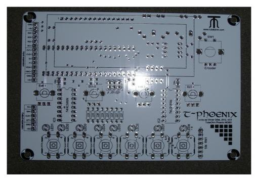
It has parts on both sides, but there's no overlap between the two regions, so when there's parts on one side, there won't be much action on the other side! The LCD has to be soldered last, since it will cover the ATMega644p pins. Otherwise you can start from whichever side you prefer.
