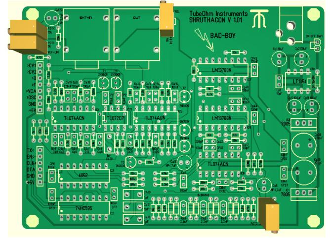
Please contact your IC's to IC socket !!!!!!Solder the sockets first !! 1x LT 1054 pay attention to the label. Mark right !!! 3x TL 073 Mark left 2x LM 13700 Mark left 1x TL 072 Mark left 1x CD 4052 Mark left 1x 74HC 595 Mark left SW 1 for on/off switch , or short it 1x Arduino header 8 pol 1x Arduino header 6 pol 1x 9V Buchse
