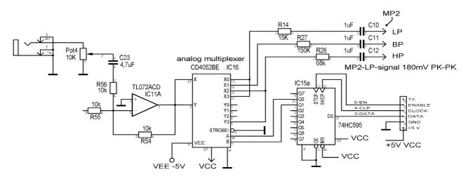
The control of the 4052 is performed by the 74HC595. This gets its data directly from the ATMEL of the motherboard.
