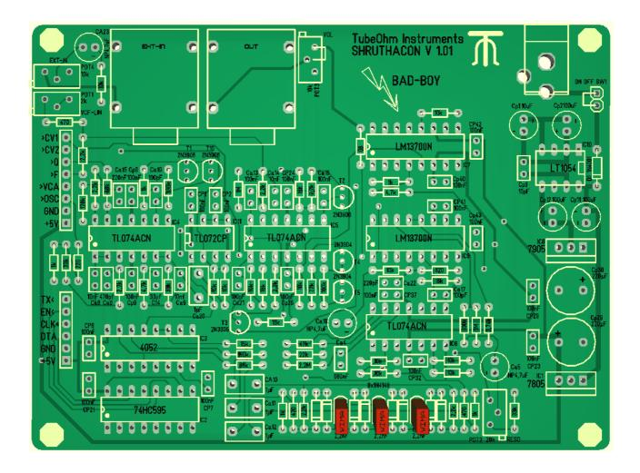
Now all components should be fitted. Before we use now the IC's we do a test of the power supply.
