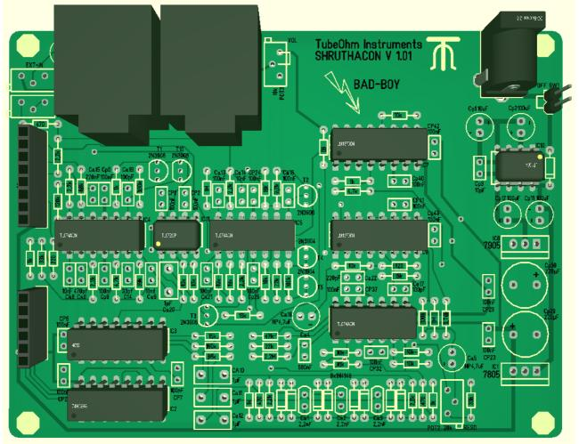
Please only solder the socket. The ICs are inserted after the test of the power supply.
