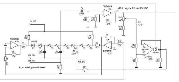
How it works? Well, let's see here ... diode1 to diode 8. These diodes are between the outputs of two operational amplifiers.
