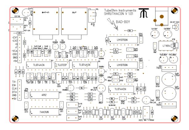
First, we assemble and solder on the PCB all the resistors as follows.
