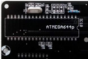
Add a 10k resistor (brown, black, black, red) near the ATMega (it pulls up the RST line of the MCU). Add the 20 MHz crystal.
