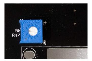
Add the 5k adjustable resistor used for LCD contrast adjustment (the photo shows that it is called R47,but it has been renamed R36 in later revisions of the board).
