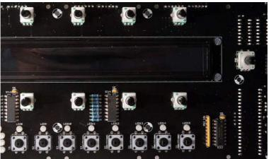
Add the 8x 10k linear pots, the encoder, and the 8x switches.
