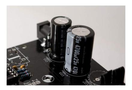
Add the two big capacitors (2200 $\mu$ F and 4700 $\mu$ F) used in the rectifier. Check and double-check their polarity.
