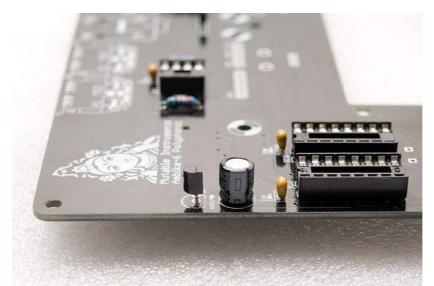
Add the MCP1700 3.3V regulator and the 100µF capacitor adjacent to it. I used here a short capacitor but the one that comes with the kit might be taller.
