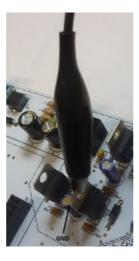
If the motherboard is connected to the 12 Volt power supply - don't forget to bridge the Power Switch K11, the LED's should turn on and the following voltages should be measured.
