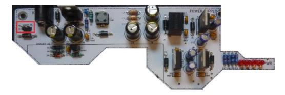
And now you can check the power supply immediately. To do this the POWER SWITCH must be short-circuited. Either with the 15 cm long cable - or profan with a jumper - if you have soldered the pin header.
