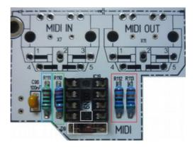
All jacks/MIDI, audio are soldered in at the very end because the board has to be turned several times and because the jacks interfere.
