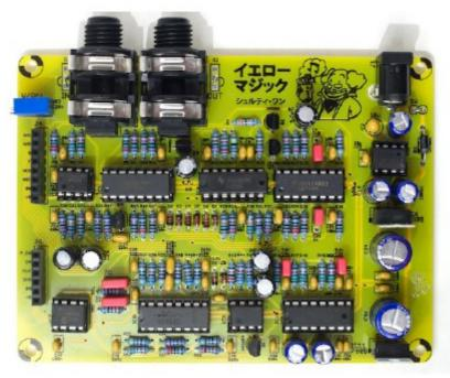
This filter boards combines a raw OTA-C 2-pole filter, combined with a classic lo-fi delay.
