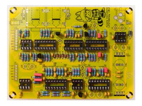
Add the 4x 2N3906 transistors, and the 2N3904 transistor. Beware of their polarity!
