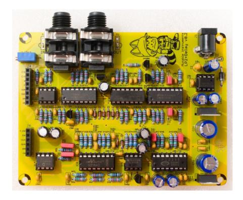
The last step consists in tuning the filter, to make sure that the cutoff frequency of the filter follows a musical scale: increasing the cutoff setting on the Shruthi by 12 (or playing a note 1 octave = 12
