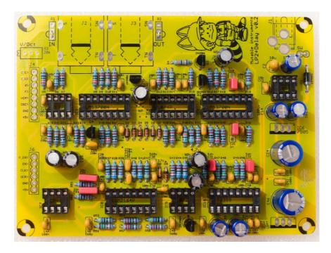
Add the electrolytic capacitors. The 6x 4.7uF capacitors are not polarized (a + and – are silkscreened on the PCB, don't bother with those). The 5x 100uF and 2x 220uF capacitors are polarized. The white stripe on the edge of the capacitor indicates the minus lead (which is also the shortest one).
