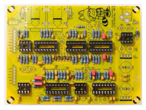
Add the film capacitors (2x 33nF, 2x 1nF, 2x 6.8nF or 5.6nF). They are clearly labelled with their value, and are not polarized.
