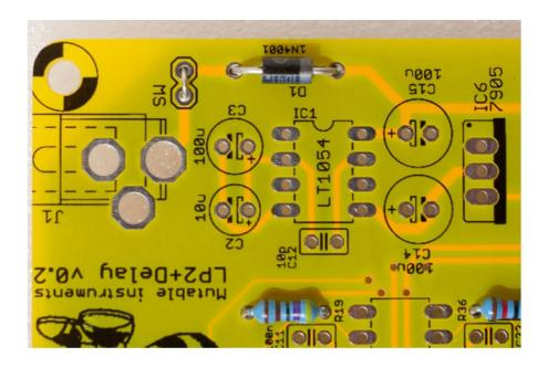
Add the polarity protection diode (1N4001 or 1N4004). It is polarized.
