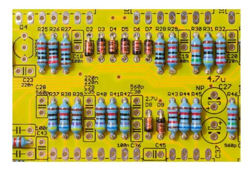
Add 6x 1N4148 diodes. They are polarized, make sure that the black ring follows the pattern silkscreened on the PCB. Add 2x 2.4V Zener diodes (this photo of an older board shows 2.7V, but the right value is 2.4V). They are polarized too.
