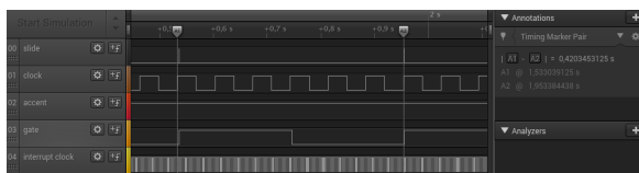
Fig. 6. Step duration of 6 clocks. 3 clocks on and 3 clocks off.
