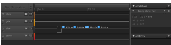
Fig. 19. Closeup of the 8.75µs slide latch.
