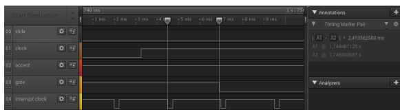
Fig. 4. Latency between interrupt clock and gate off.
