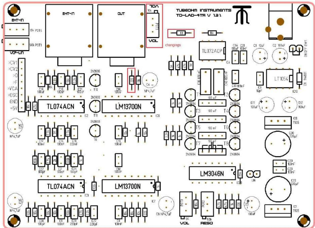
The solder instruction V 1.31 is nearly the same like in V 1.3 but with three changes. First, there is a 10K vol pot, second, we removed one 10 K resistor and third, we replace a 1K ohm against a 220 ohm, so we reduce the output volume.
