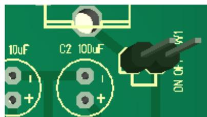
Both pins are for a POWER ON/OFF switch. If you don't want to connect a power switch, just bridge it.
