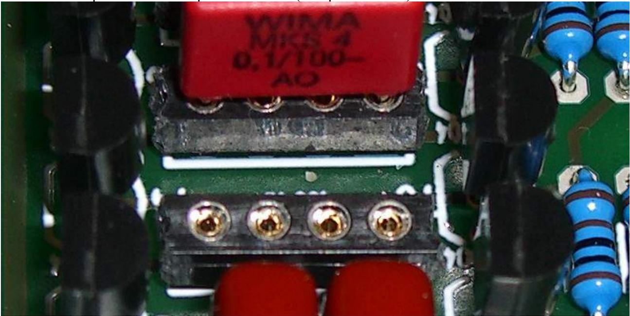
The sockets for the capacitors is a 'CAN do' not a 'MUST do' ! You can simply solder 4 x 100 nF capacitors !
