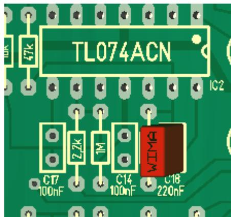
Than the ladder capacitors. We recommend 4x 100 nF for a wide frequency range. But you can change the value to 150 nF or 120 nF. If you wish to experiment, we suggest that you build in 4 sockets for the capacitors. Simply use a precision IC socket and cut 4 connectors. You can than push different capacitors into it. ( see photo below)
