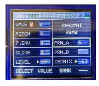
The new parameter on the right-hand side is **PRM\_A**. This regulates from a sine wave to a sawtooth.
