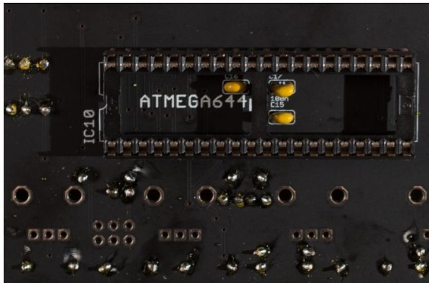
Flip the board and solder a socket on the back for IC10.
