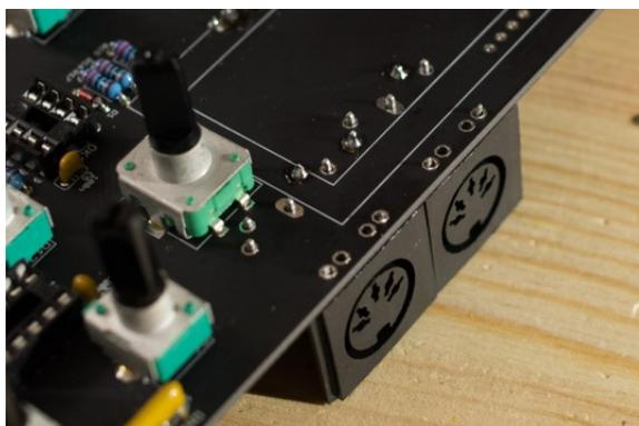
Add the MIDI connectors. It is recommended to solder only one leg (as shown on the photo) - if necessary adjust their alignment; and once everything is okay, finish soldering all pins.
