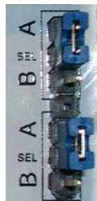
A voicecard can either be inserted into the Ambika motherboard ; or stacked on top of another voicecard. In the former case, the two jumpers must be set to the A position. In the later case, the two jumpers must be set to the B position.
