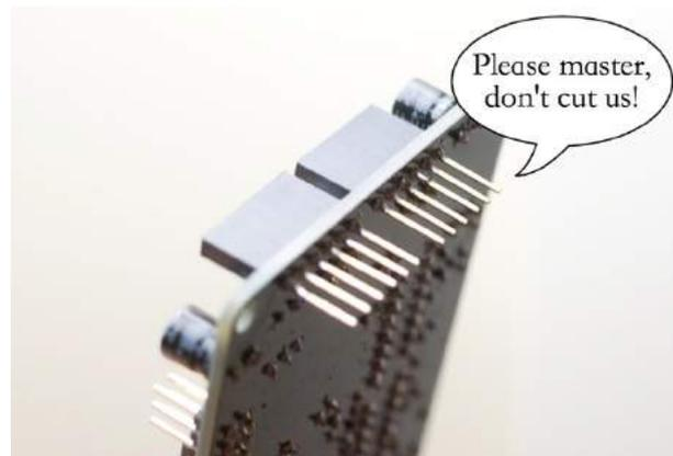
Do not trim the leads of the board stacking connectors. The voicecard is stacked on top of the motherboard or of another voicecard, so the 6 leads of the 1×6 connectors should be kept long. This is the same stacking approach as the Arduino “shields”.
