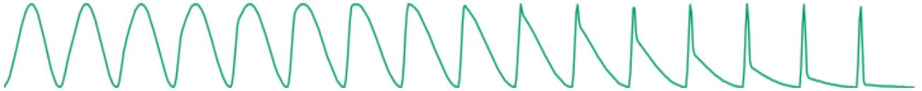
This waveform uses phase distortion to recreate a low-pass filtered sawtooth by progressively “pinching” the phase of a sine wave. The parameter controls the brightness of the sound: from a sine wave to a sawtooth, then from a sawtooth to a sawtooth gone through an ugly transistor amp. Good for dirty bass guitar sounds or clavinet.
