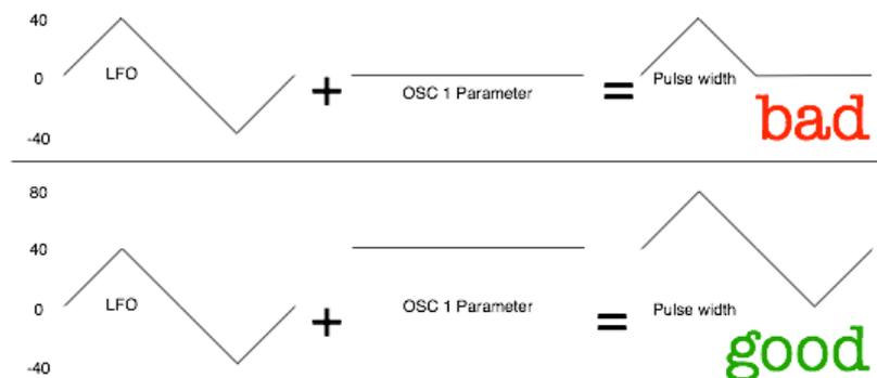
LFOs, pitch-bend and MIDI note number modulations are bipolar. If you are used to electronics/Modular speak, it is equivalent to say that the LFOs are always “AC-coupled” instead of “DC-coupled”.
