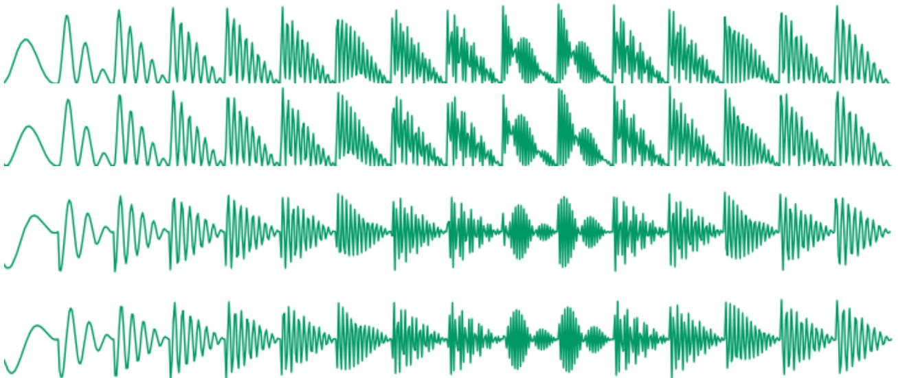
This waveform family directly simulates the sound of a sawtooth wave processed by a low-pass, peaking, band-pass, or high-pass resonant filter. The parameter controls the cutoff frequency of the filter.
