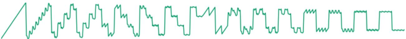
A palette of 8-bits sounding waveforms obtained by applying bitwise operations to a basic sawtooth wave (something now known as "biscuiting").
